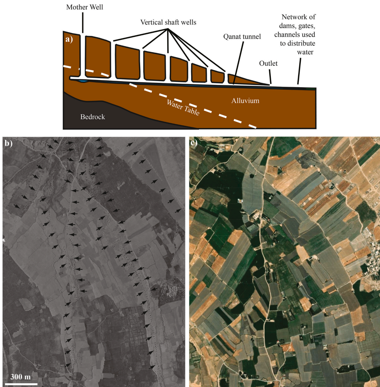
Fig. 7. a) Schematic qanat cross section (modified after English, 1968). b) Aerial photo (from National Cartographic Center of Iran – 1973) showing qanats in the Firuzabad plain (the black arrows indicate the paths of 6 different qanats ); the aligned dark dots correspond to vertical shaft wells. c) Present day satellite image of the same area represented in Fig. 7b which shows how the cultivated lands covered the traces of the pre-existing qanats (from Esri, Maxar, GeoEye, Earthstar Geographics, CNES/Airbus DS, USDA, USGS, AeroGRID, IGN, and the GIS User Community).
